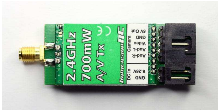
Fig 1. Top side of ImmersionRC 700mW 2.4GHz audio/video transmitter.
